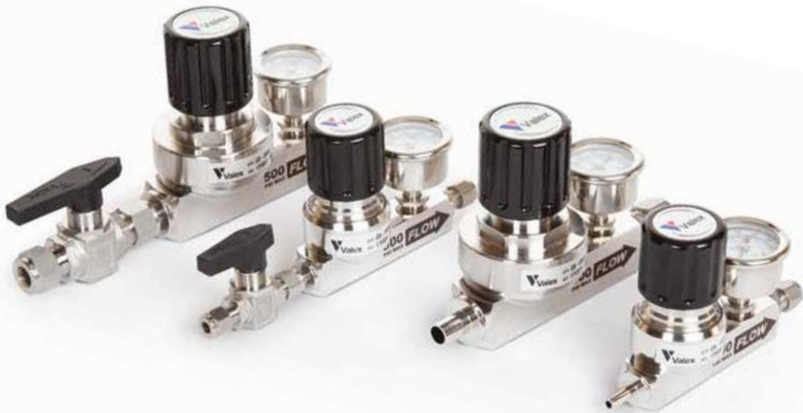
Bulk gas sticks typically consist of the marriage of three components: a shutoff valve, a pressure control regulator, and gauge. Our CFOS gas stick combines these components into a singular, simple-to-use, integrated device.
